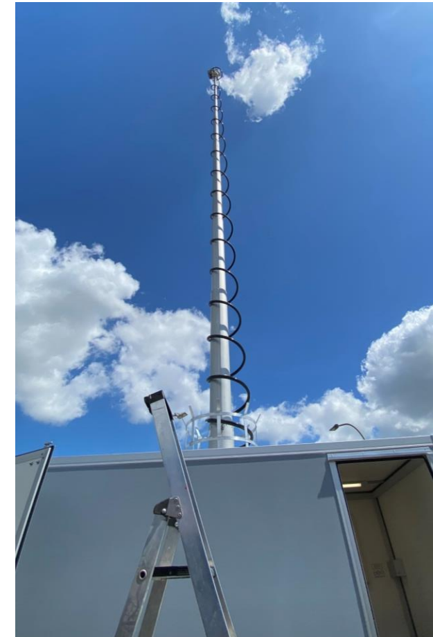
Hydraulic Antenna (max. 16 m height)
